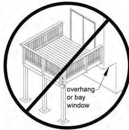
Figure 18. No Attachment to House Overhang with Ledger.
